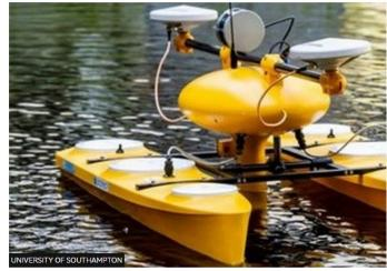
Researchers are using an autonomous surface vehicle to survey the seagrass meadows at Studland
